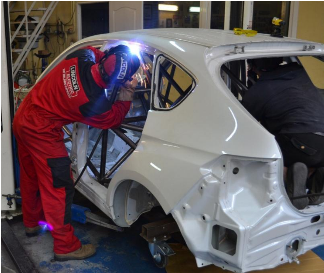
Speedtec 200C, Linc Gun LB150-3m, Acier & Inox, fil de 0,8mm, Ar/CO 2
